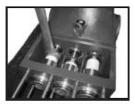
4. Separate plunger connection (36A) from crosshead (25) by means of two open-end wrenches (size 22 and 27). Pull seal sleeves (39) out of their fittings in the crankcase.
